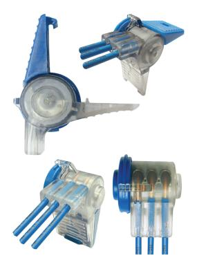
Pro-Trace TW Connector is used for underground splices or connections for tracer wire systems, and other applications not exceeding 300 Volts. The silicone filled connector is used to splice or branch-off multiple tracer wires to maintain continuity and provides corrosion-proof protection from underground elements.
